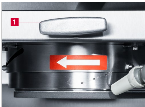
Figure 7-7 Loosening the grinding wheel
