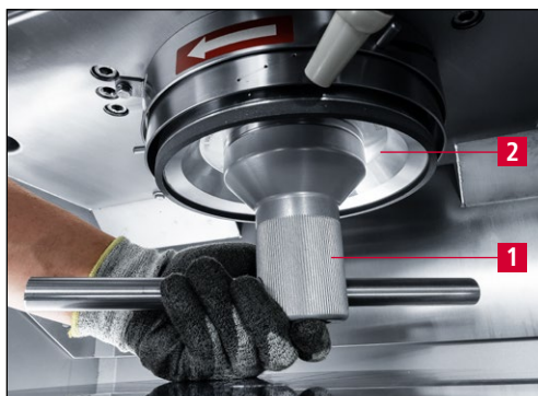
Figure 7-8 Loosening the grinding wheel
