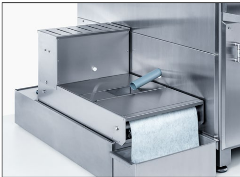
Figure 6-1 Filling the belt filter coolant unit
