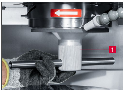
Figure 7-9 Replacing the grinding wheel
