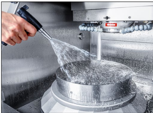
Figure 9-1 Rinsing the rotary table
