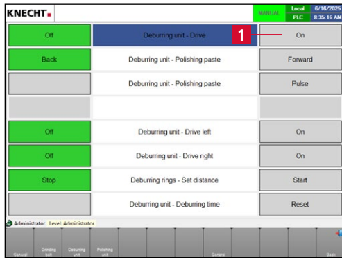
Figure 6-9 Manual functions "Deburring unit"
