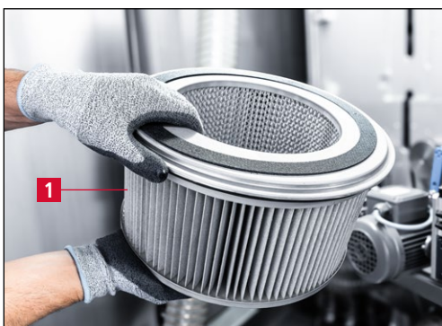
Bild 9-5 Cleaning the filter cartridge
