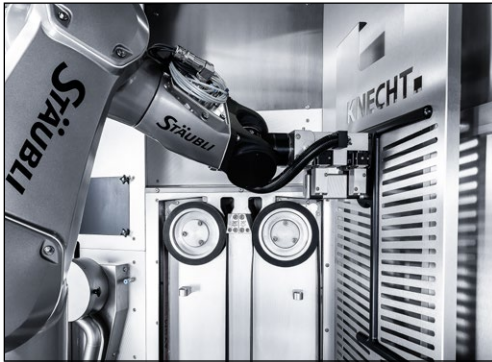
Figure 7-10 Closing the belt protection hood
