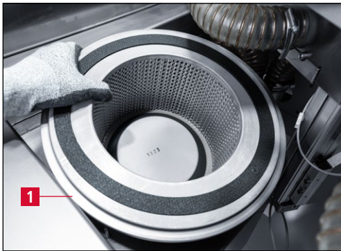
Figure 9-4 Removing the filter cartridge
