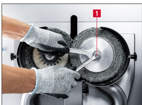
Figure 7-28 Unscrewing the right clamping nut
