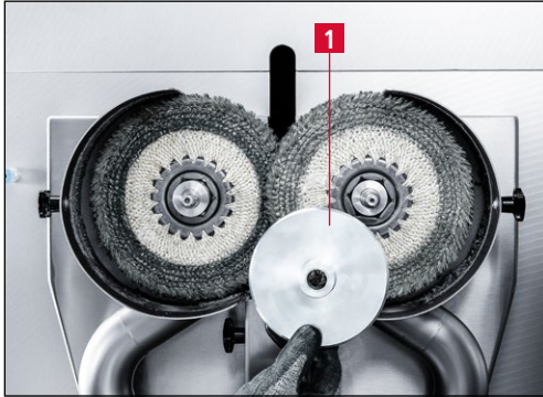
Figure 7-29 Removing the flange washer
