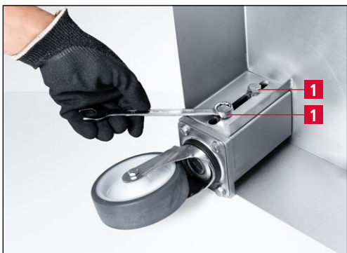
Figure 5-2 Adjusting the steering rollers
