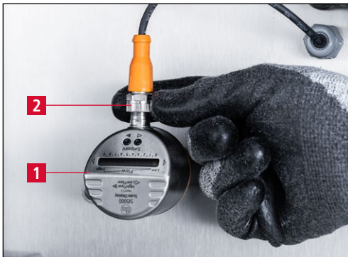
Figure 9-6 Unplugging the flow monitor
