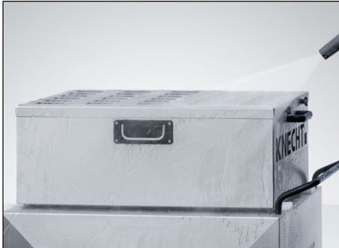
Figure 9-9 Cleaning the knife magazines
