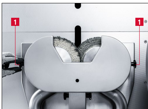
Figure 7-22 Loosening the star handles
