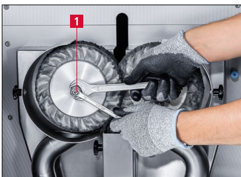
Figure 7-45 Unscrewing the left clamping nut
