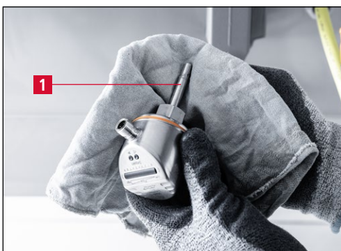
Figure 9-8 Cleaning the measuring probe
