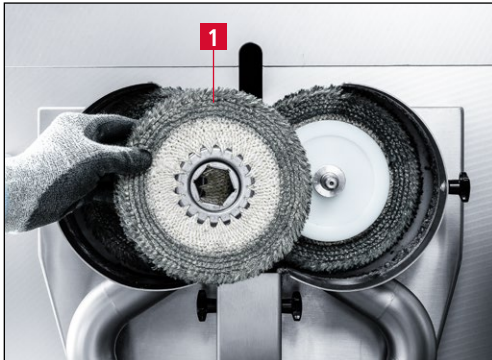
Figure 7-30 Removing the used deburring ring
