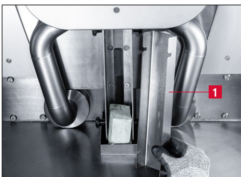
Figure 7-59 Removing the cover
