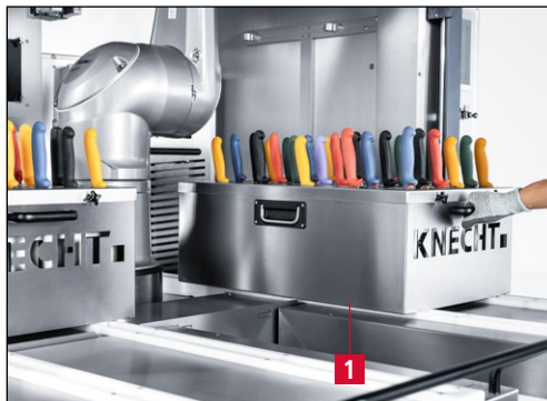
Figure 7-4 Moving the knife magazines into the grinding machine
