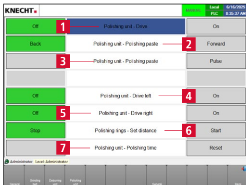
Figure 8-11 Manual functions "Polishing unit"
