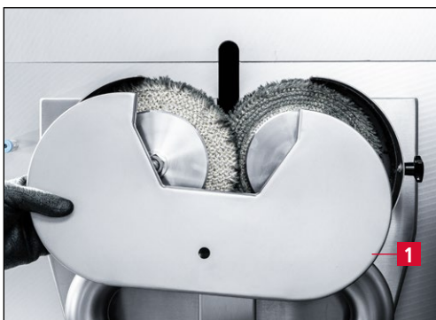
Figure 7-22 Removing the protection hood
