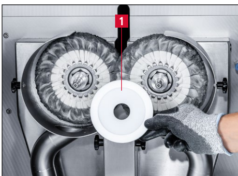
Figure 7-48 Removing the intermediate flange
