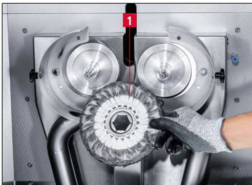
Figure 7-50 Replacing the polishing rings
