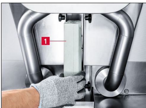
Figure 7-56 Replacing the polishing paste
