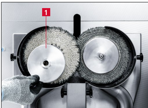
Figure 7-25 Removing the flange washer
