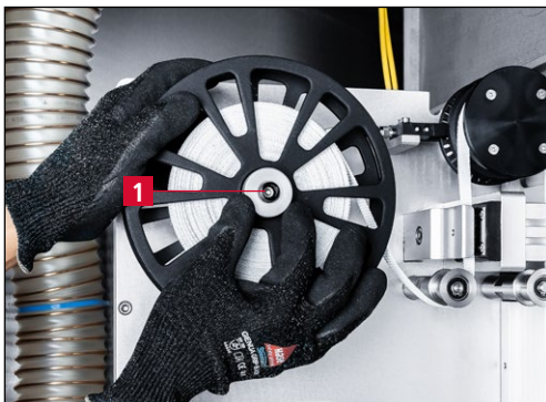
Figure 7-62 Removing the used test medium
