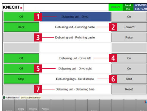
Figure 8-10 Manual functions “Deburring unit”
