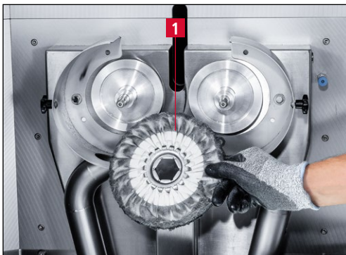
Figure 7-51 Replacing the polishing rings
