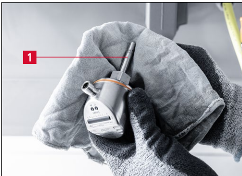
Figure 9-8 Cleaning the measuring probe
