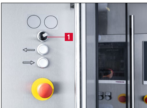
Figure 7-2 Control panel rotary magazine
