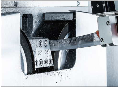
Figure 7-7 Grinding hand knives
