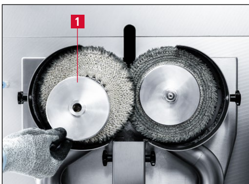
Figure 7-26 Removing the flange washer
