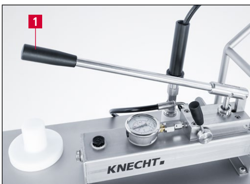
Figure 5-5 Building up hydraulic pressure
