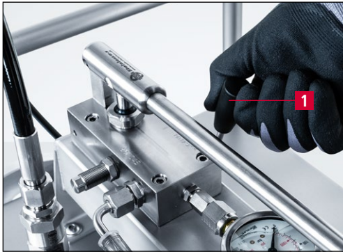
Figure 5-26 Closing the pump valve
