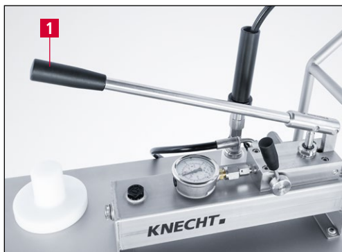
Figure 5-12 Building up hydraulic pressure
