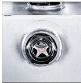
Inspection glass with correct oil level
