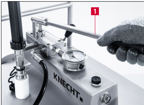
Figure 5-27 Building up hydraulic pressure
