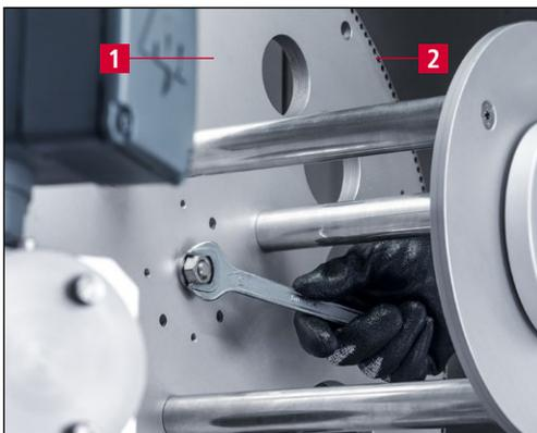
**Figure 7-5** Mounting the SP 116 Cam plate
