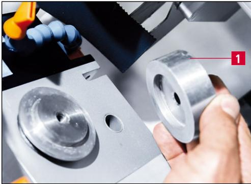
**Figure 7-23** Intermediate flange
