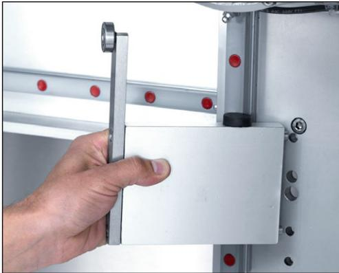
**Figure 7-4** Mounting the Z-coupling
