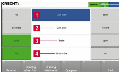
Figure 8-13 Manual functions “Cam plate”
