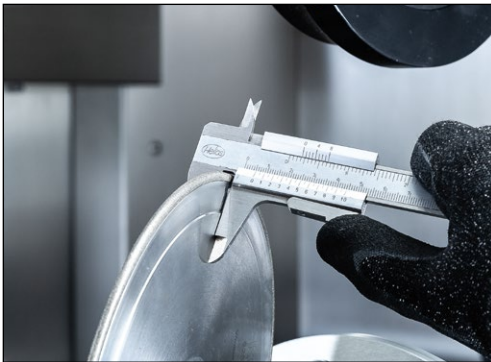
Figure 7-56 Measuring the thickness of the profiling wheel
