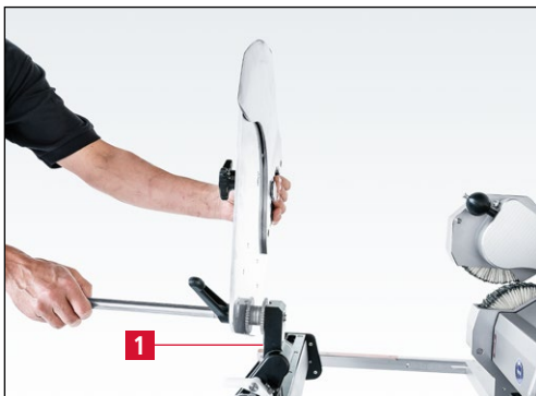
Figure 7-52 Cutter knife swiveled back and secured
