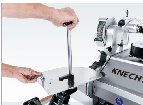
Figure 7-129 Polishing the knife bale
