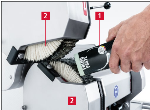
Figure 7-122 Applying the polishing paste
