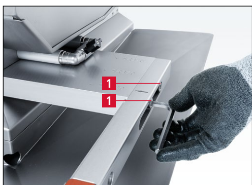
Figure 7-30 Loosen the M10 screws
