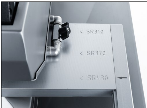
Figure 7-28 Set position of the grinding and polishing unit
