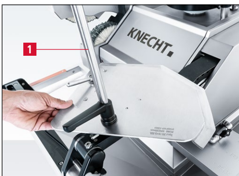
Figure 7-135 Swiveling the cutter knife to the next cutting segment and grind
