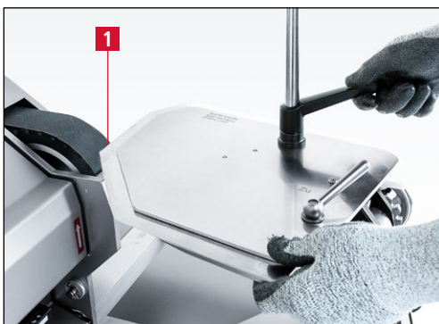
Figure 7-114 Aligning the knife on the grinding belt
