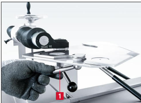
Figure 7-80 Locking the knife on the grinding plate
