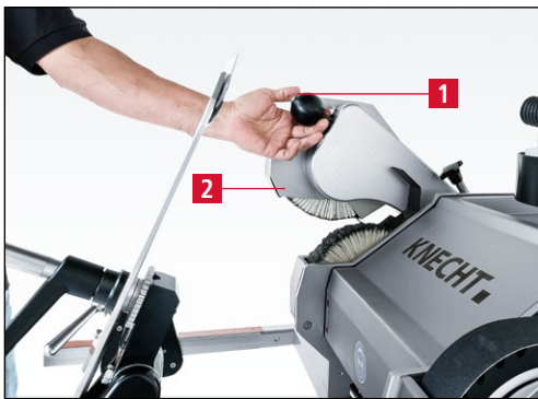
Figure 7-131 Moving the upper polishing unit into the working position
