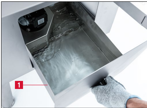
Figure 6-1 Filling the water tank
