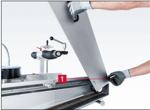
Figure 7-149 Closing the belt protection hood
