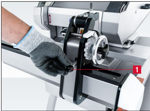
Figure 7-33 Locking the carriage in position
