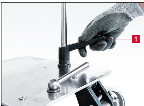
Figure 7-113 Loosening the grinding lever
