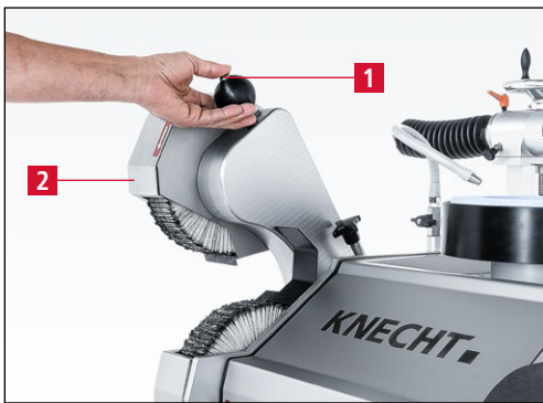
Figure 7-64 Moving the upper polishing unit into the working position
