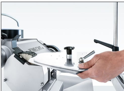
Figure 7-62 Polishing the knife bale
