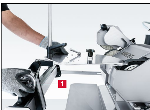
Figure 7-47 Moving the grinding unit to the grinding belt
