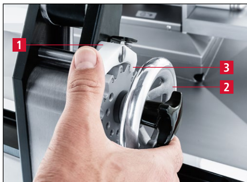
Figure 7-49 Bringing the grinding unit into grinding position "1"
