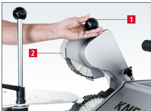
Figure 7-127 Swiveling the upper polishing unit upward
