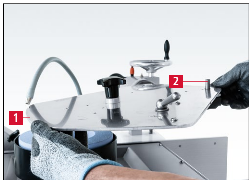
Figure 7-8 Mounting the grinding plate
