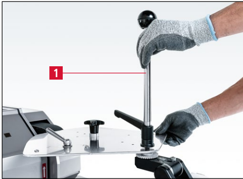
Figure 7-38 Slightly tightening the grinding lever
