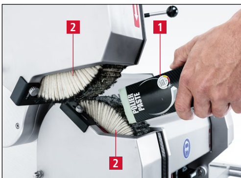
Figure 7-54 Applying the polishing paste
