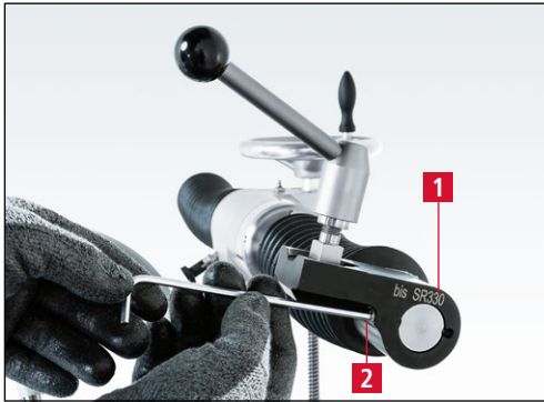
Figure 7-70 Fitting the mounting head
