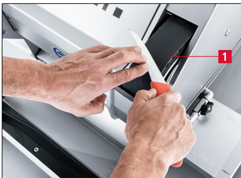
Figure 7-136 Grinding hand knives
