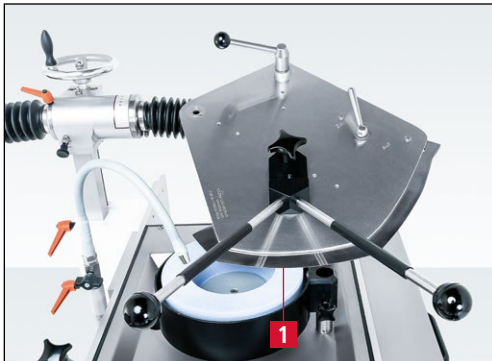
Figure 7-19 Knife position on the grinding wheel
