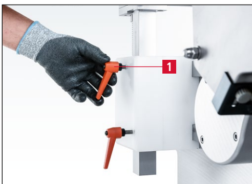
Figure 7-21 Loosening the clamping lever
