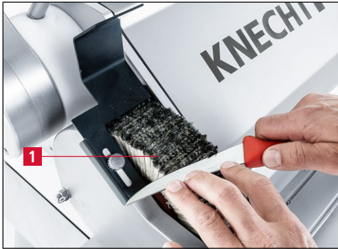
Figure 7-138 Deburring and polishing hand knives
