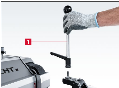
Figure 7-99 Removing the grinding lever
