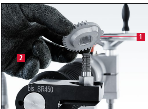
Figure 7-7 Inserting the function disc
