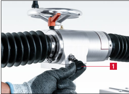
Figure 7-73 Engaging the locking bolt
