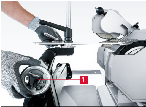
Figure 7-112 Moving the grinding unit to the grinding belt
