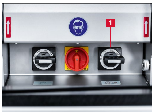
Figure 7-128 Switching on the grinding machine
