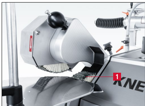
Figure 7-124 Knife rests on the finned brush
