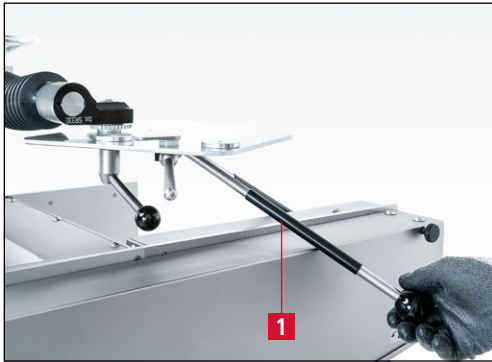
Figure 7-78 Swiveling the grinding plate to the rear
