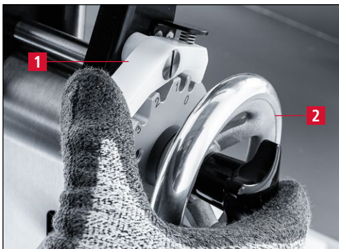
Figure 7-110 Bringing the grinding unit into adjustment position "0"
