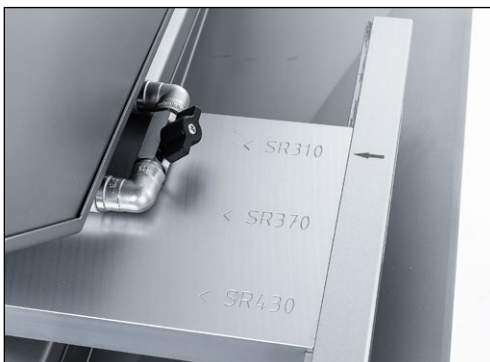
Figure 7-94 Set position of the grinding and polishing unit
