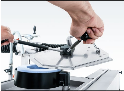
Figure 7-92 Swiveling the cutter knife to the next cutting segment and grind
