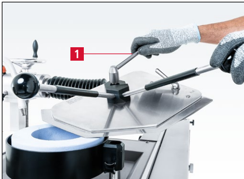
Figure 7-84 Loosening the clamping lever
