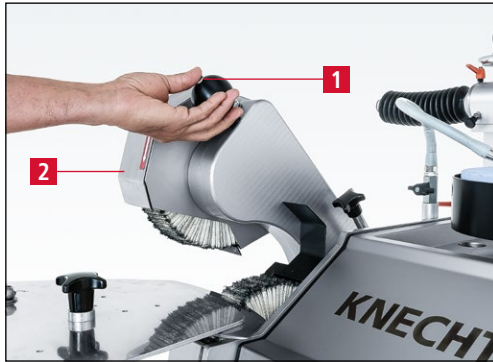
Figure 7-60 Swiveling the upper polishing unit upward
