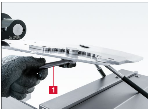
Figure 7-18 Locking the knife on the grinding plate
