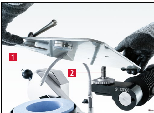
Figure 7-75 Mounting the grinding plate
