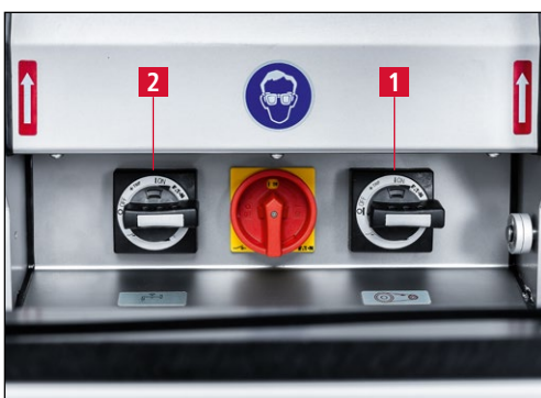
Figure 7-123 Switching off the grinding machine
