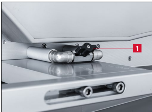
Figure 3-5 Coolant dosing for wet-grinding belt
