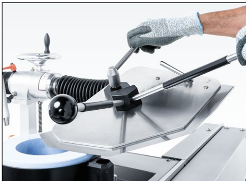
Figure 7-85 Aligning the knife on the grinding wheel
