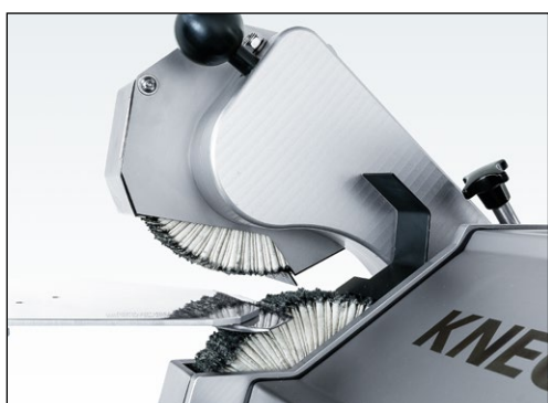
Figure 7-125 Distance between finned brushes approx. 20 mm
