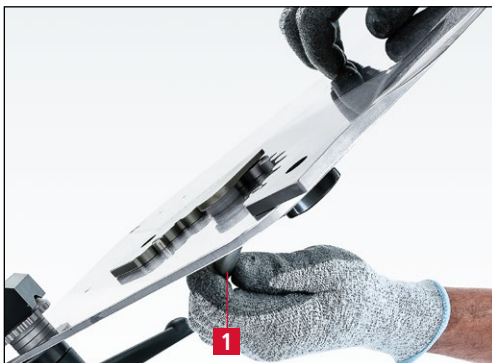
Figure 7-42 Locking the knife on the grinding plate
