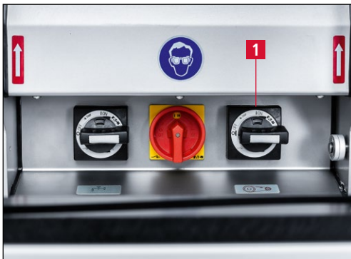
Figure 7-133 Switching off the grinding machine
