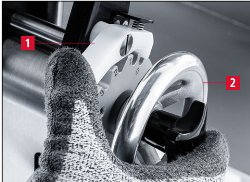
Figure 7-45 Bringing the grinding unit into adjustment position "0"
