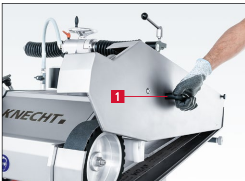
Figure 7-146 Opening the belt protection hood
