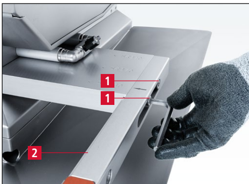
Figure 7-96 Loosen the M 10 screws
