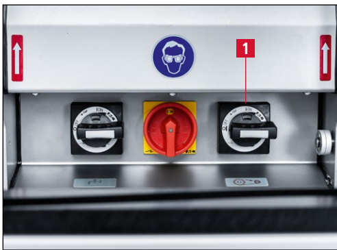
Figure 7-61 Switching on the grinding machine
