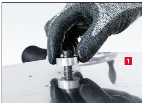
Figure 7-10 Removing the spacer disc
