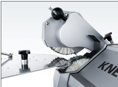
Figure 7-58 Distance between finned brushes approx. 20 mm
