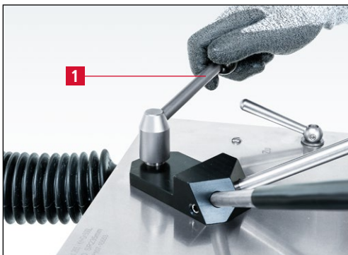
Figure 7-86 Tightening the clamping lever
