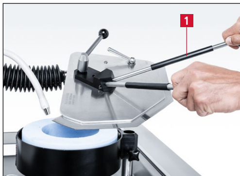
Figure 7-90 Grinding linear cutter knives
