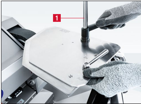
Figure 7-115 Tightening the grinding lever
