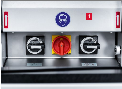
Figure 7-66 Switching off the grinding machine
