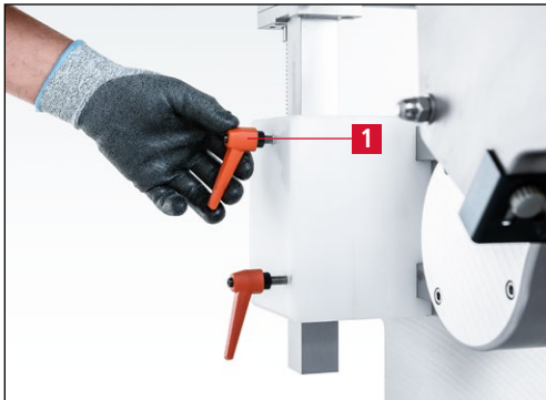
Figure 7-87 Loosening the clamping lever
