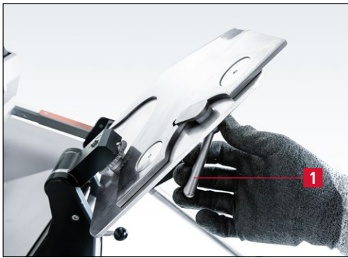
Figure 7-107 Locking the knife on the grinding plate
