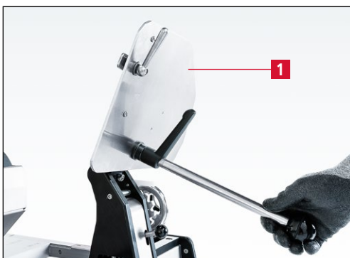
Figure 7-105 Swiveling the grinding plate backward
