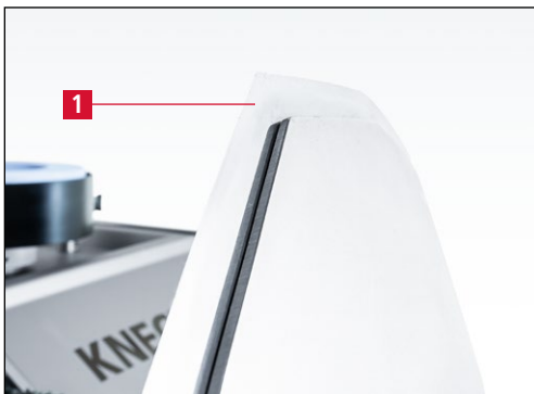
Figure 7-134 Checking the knife sharpness
