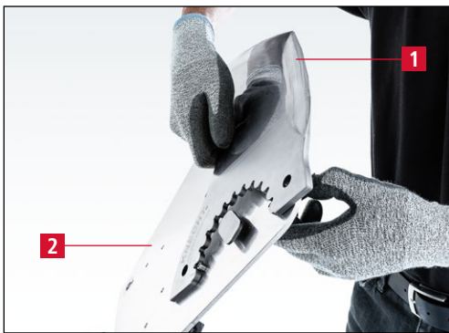
Figure 7-41 Clamping the knife onto the grinding plate
