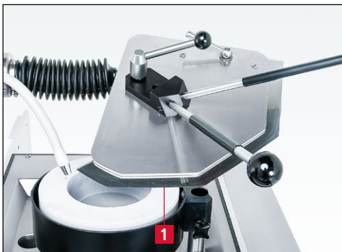
Figure 7-82 Knife position on the grinding wheel
