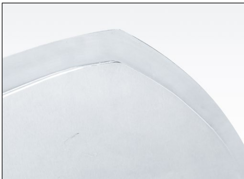
Figure 7-67 Checking the knife sharpness
