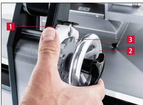
Figure 7-117 Bringing the grinding unit into grinding position "1"
