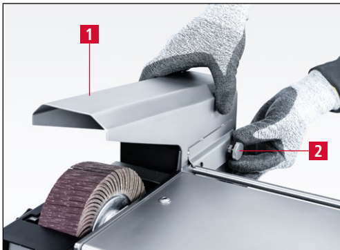
Figure 6-1 Removing the splash guard
