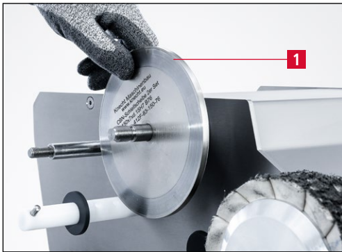
Figure 6-7 Fitting the CBN grinding wheel
