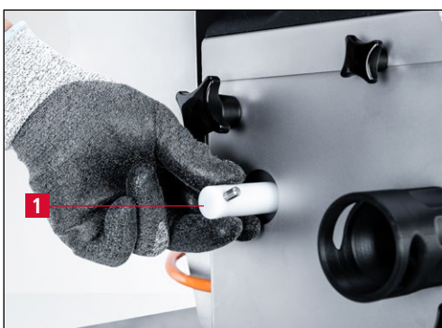
Figure 7-2 Adjusting the water nozzle
