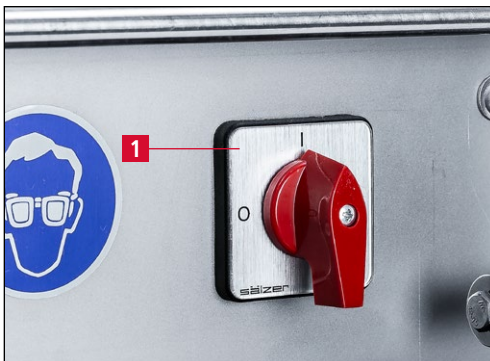
Figure 7-1 Switching on the sharpening machine
