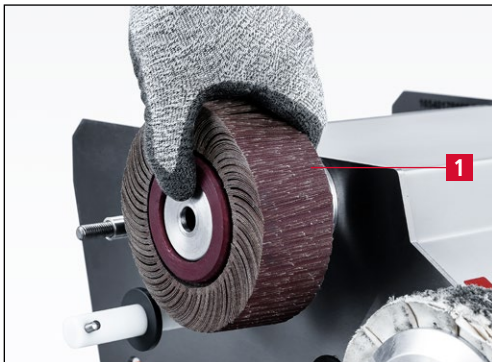
Figure 6-4 Removing the finned-grinding wheel
