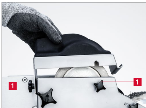
Figure 7-7 Removing the grinding attachment
