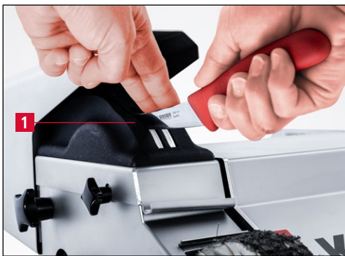
Figure 7-3 Sharpening the hand knife
