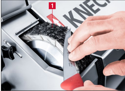
Figure 7-5 Deburring and polishing the hand knife
