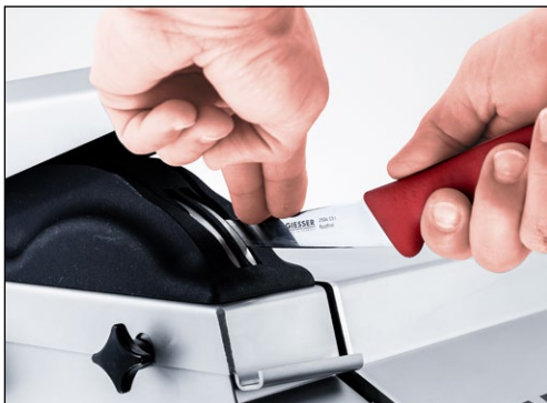
Figure 7-4 Sharpening the hand knife
