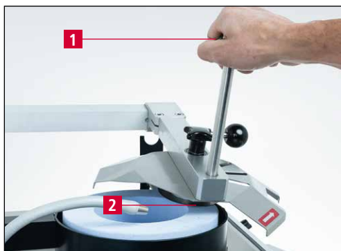
Figure 7-11 Grinding the circular knife
