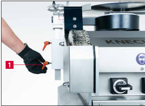
Figure 7-19 Adjusting the circular knife grinding attachment
