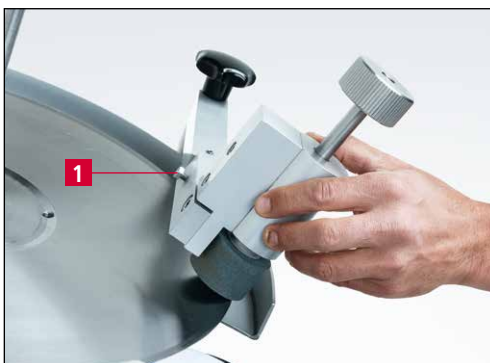
Figure 7-25 Swiveling the deburring arm
