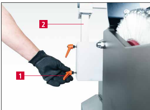
Figure 7-6 Adjusting the circular knife grinding attachment
