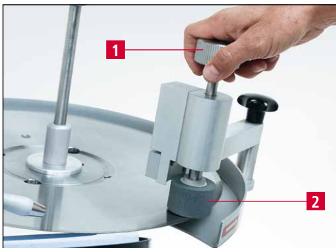
Figure 7-24 Deburring the circular knife
