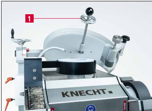
Figure 7-13 HV 205-2 circular knife grinding attachment
