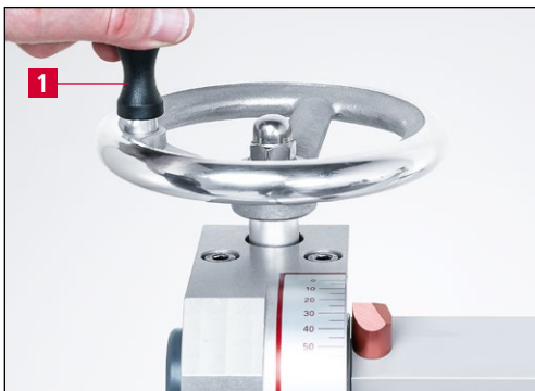
Figure 7-19 Reducing the grinding angle (convex grinding)
