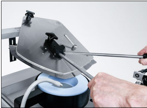
Figure 7-20 Swiveling the cutter knife to the next cutting segment and grind
