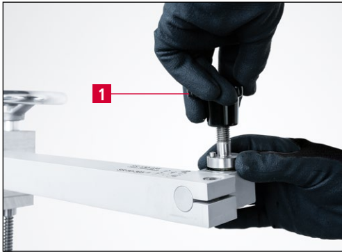
Figure 7-2 Removing the star handle
