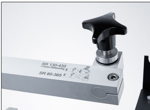
Figure 7-1 Checking the position of the mounting head
