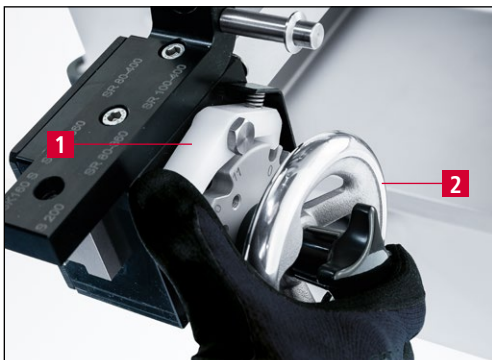
Figure 9-12 Bringing the grinding unit into adjustment position "0"
