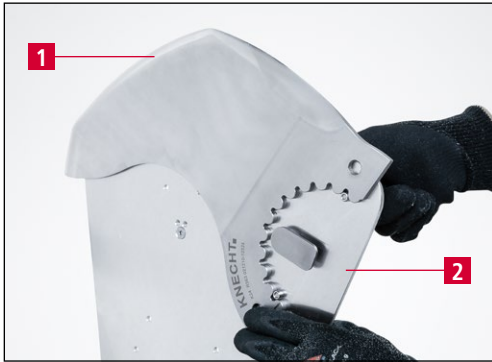
Figure 9-8 Clamping the knife onto the grinding plate
