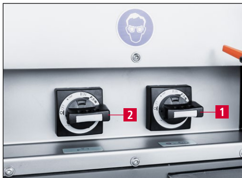
Figure 9-15 Switching on the grinding machine and coolant unit
