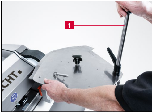
Figure 9-21 Swiveling the cutter knife to the next cutting segment and grind
