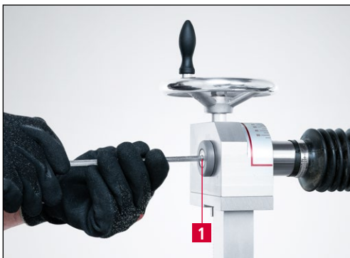
Figure 6-1 Removing the HV 203 Universal grinding arm
