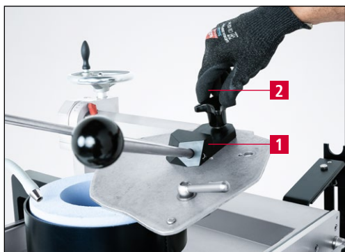
Figure 7-9 Mounting the grinding lever on the locating bolt
