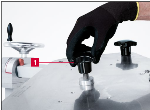
Figure 7-6 Removing the star handle
