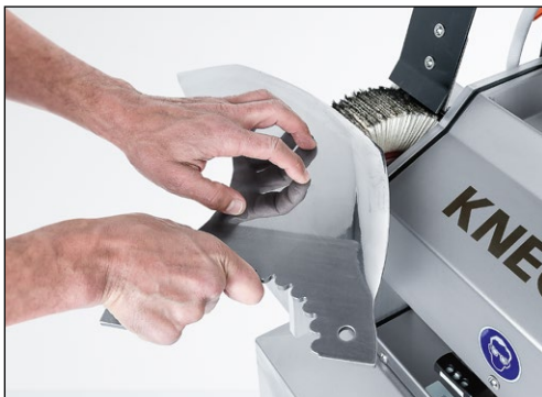
Figure 9-22 Deburring and polishing the cutter knife on the finned brush
