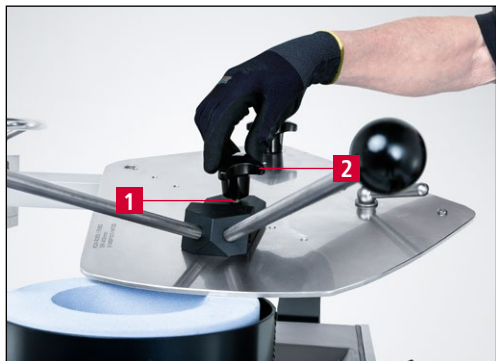
Figure 7-8 Mounting the grinding lever on the grinding plate
