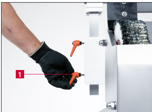
Figure 7-14 Adjusting the knife to the center of the grinding wheel
