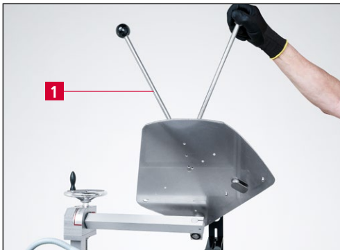
Figure 7-10 Swiveling the grinding plate backward
