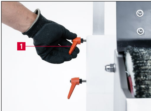
Figure 7-15 Loosening the clamping lever
