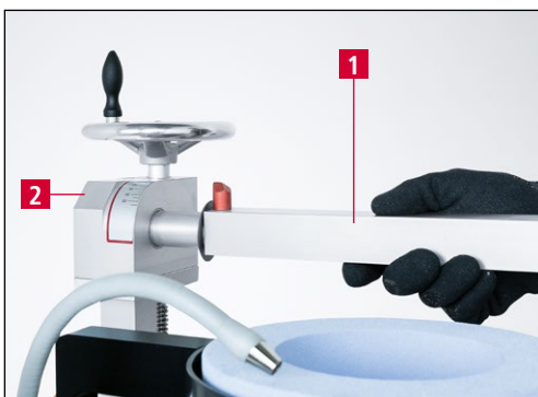
Figure 6-2 Mounting the HV 207 Swivel Arm
