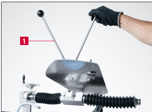
Figure 7-39 Swiveling the grinding plate backward
