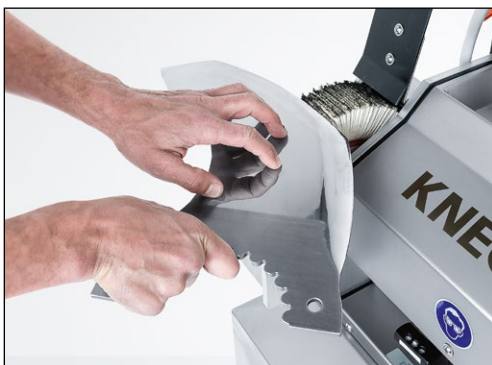
Figure 9-50 Deburring and polishing the cutter knife on the finned brush
