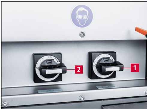
Figure 9-43 Switching on the grinding machine and coolant unit
