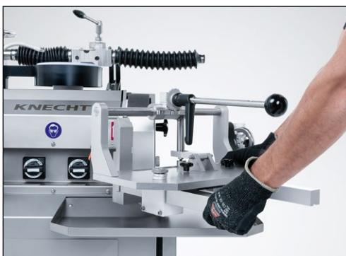
Figure 8-2 Swiveling the HV 262 into working position
