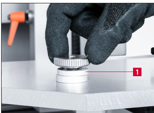
Figure 9-29 Spacer discs for adjusting grinding angle
