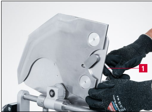
Figure 9-10 Locking the knife on the grinding plate
