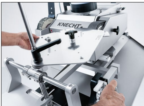
Figure 9-42 Moving the grinding unit to the grinding belt
