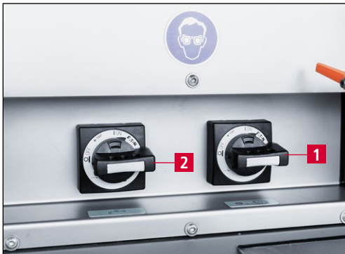
Figure 7-46 Switching on the grinding machine and coolant unit
