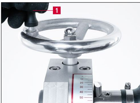
Figure 7-24 Reducing the grinding angle (convex grinding)
