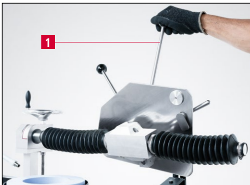
Figure 7-8 Swiveling the grinding plate backward
