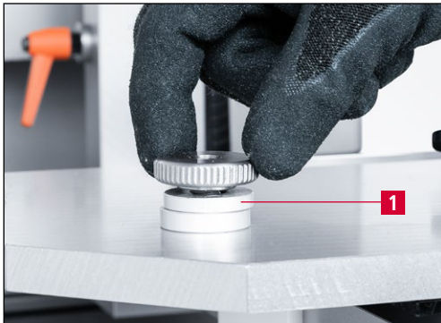
Figure 9-4 Spacer discs for adjusting grinding angle
