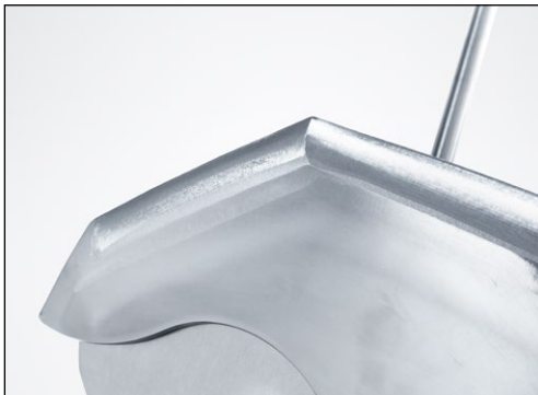
Figure 7-26 Convex pre-ground cutter knife
