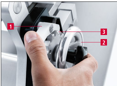
Figure 9-20 Bringing the grinding unit into grinding position "1"
