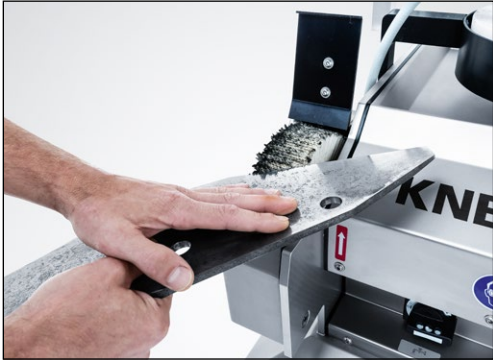
Figure 7-21 Deburring and polishing linear knives on the finned brush
