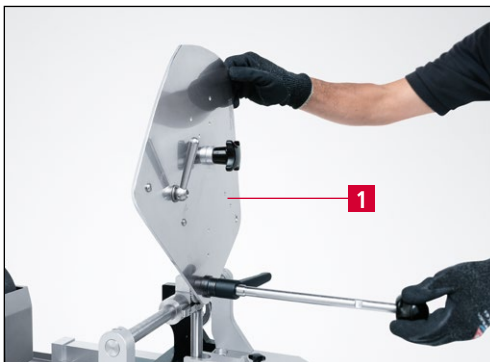
Figure 9-35 Swiveling the grinding plate backward into the anti-rotation lock
