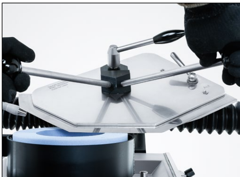
Figure 7-15 Aligning the knife on the grinding wheel
