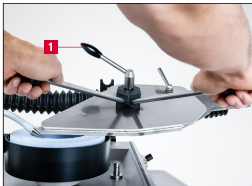
Figure 7-20 Grinding linear knives with tapered cutting edges
