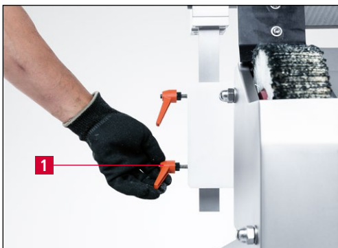
Figure 7-43 Adjusting the knife to the center of the grinding wheel
