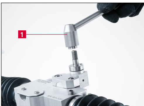
Figure 7-4 Removing the clamping lever
