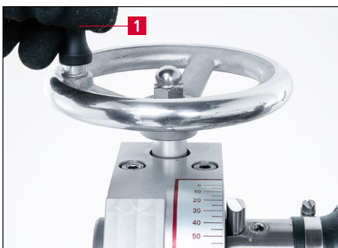
Figure 7-48 Reducing the grinding angle (convex grinding)
