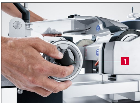
Figure 9-48 Retracting the grinding unit
