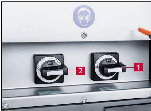
Figure 7-22 Switching on the grinding machine and coolant unit
