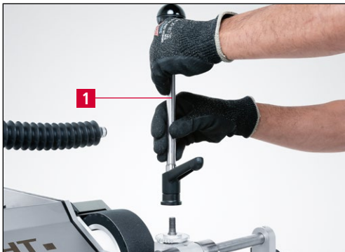
Figure 9-2 Removing the grinding lever
