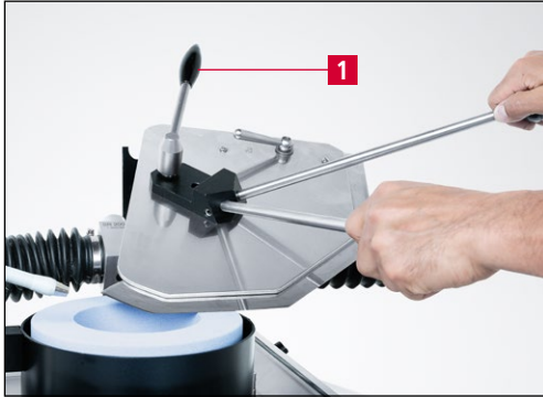
Figure 7-25 Swiveling the cutter knife to the next cutting segment
