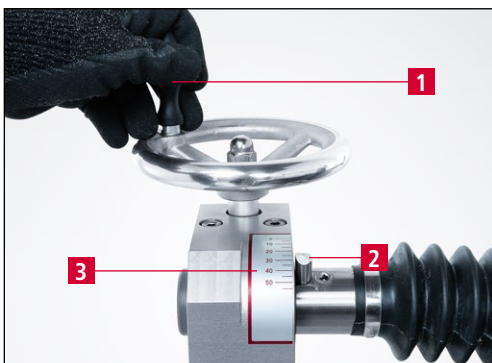
Figure 7-18 Setting the grinding angle
