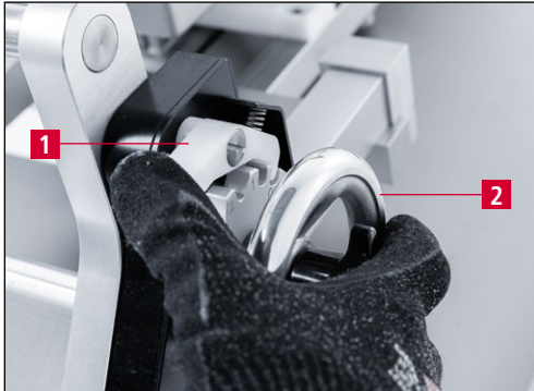
Figure 9-40 Bringing the grinding unit into adjustment position "0"
