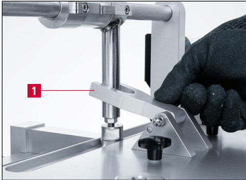
Figure 9-27 Locking the carriage
