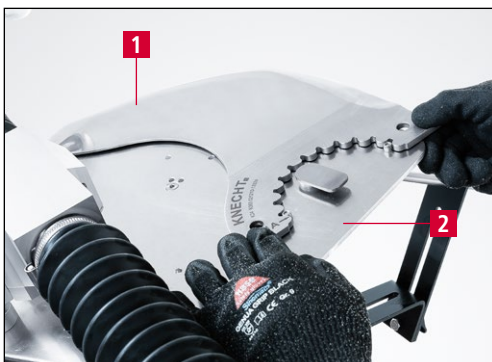
Figure 7-40 Clamping the knife onto the grinding plate
