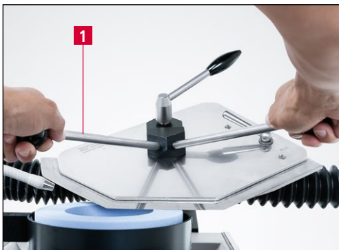
Figure 7-23 Grinding linear cutter knives
