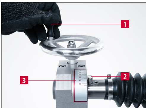
Figure 7-45 Setting the grinding angle
