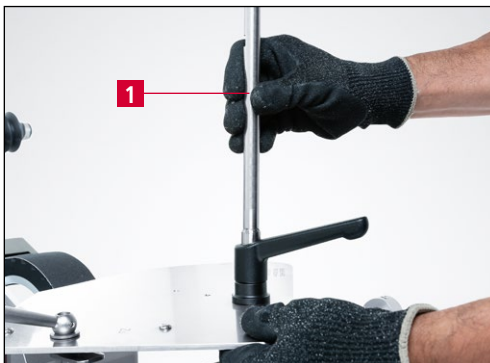
Figure 9-7 Clamping the grinding plate
