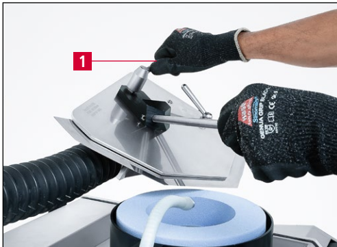
Figure 7-14 Loosening the clamping lever
