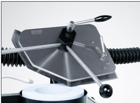
Figure 7-11 Swiveling the grinding plate forward
