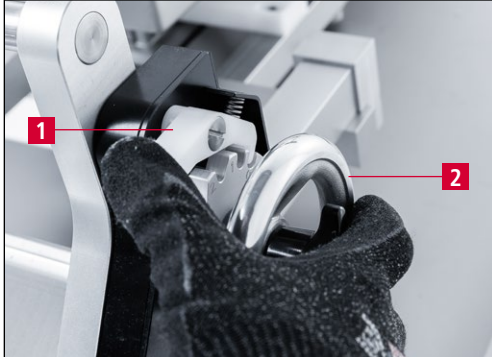
Figure 9-13 Bringing the grinding unit into adjustment position "0"
