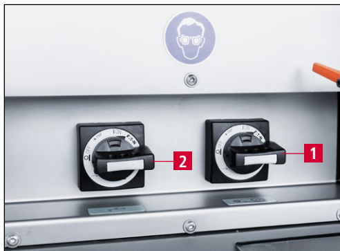
Figure 7-19 Switching on the grinding machine and coolant unit
