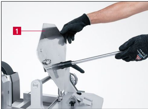
Figure 9-8 Swiveling the grinding plate backward
