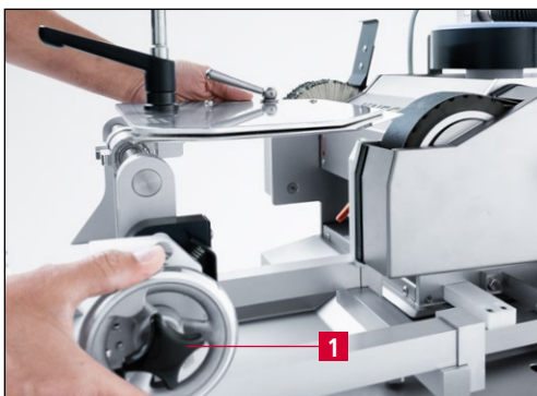
Figure 9-24 Retracting the grinding unit
