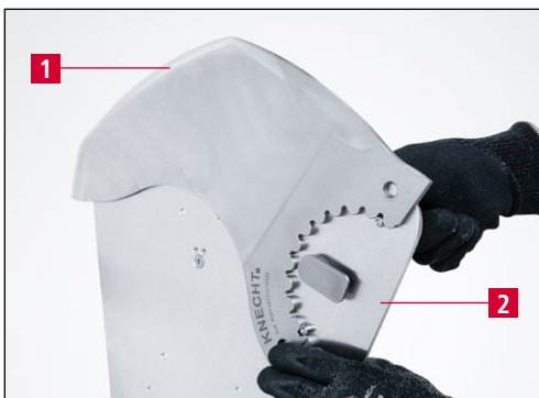
Figure 9-36 Clamping the knife onto the grinding plate
