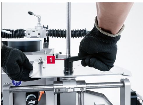
Figure 9-18 Tightening the grinding lever
