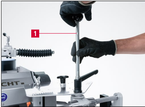
Figure 9-32 Slightly tightening the grinding lever
