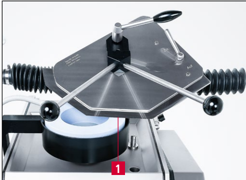
Figure 7-12 Knife position on the grinding wheel
