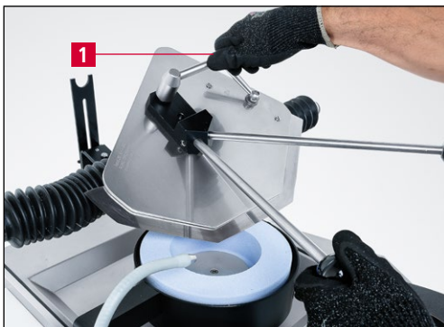
Figure 7-16 Tightening the clamping lever
