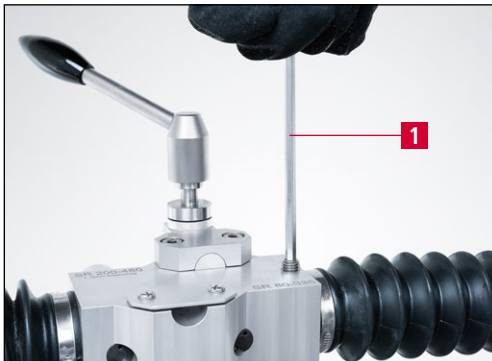
Figure 7-3 Loosening the carriage
