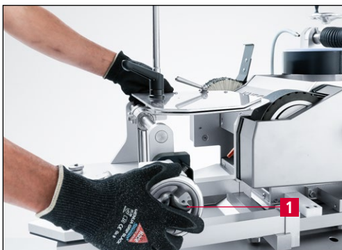
Figure 9-15 Moving the grinding unit to the grinding belt
