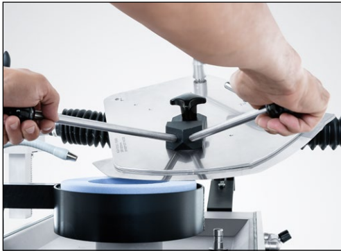
Figure 7-49 Swiveling the cutter knife to the next cutting segment
