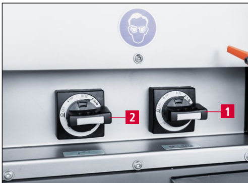
Figure 9-19 Switching on the grinding machine and coolant unit
