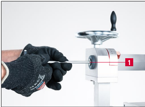
Figure 6-1 Removing the swivel arm
