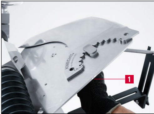
Figure 7-41 Locking the knife on the grinding plate
