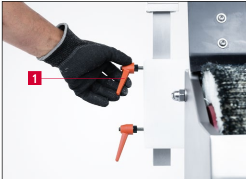
Figure 7-17 Loosening the clamping lever
