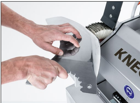
Figure 9-26 Deburring and polishing the cutter knife on the finned brush
