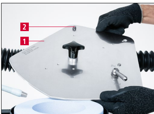
Figure 7-34 Mounting the grinding plate
