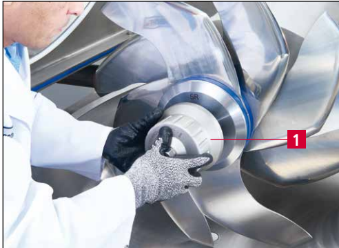
Figure 5-12 Installing the MCF 100 Mechanical spring clamping nut
