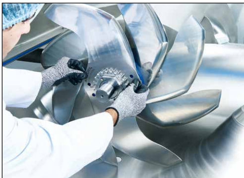
Figure 5-8 Assembling the knife package
