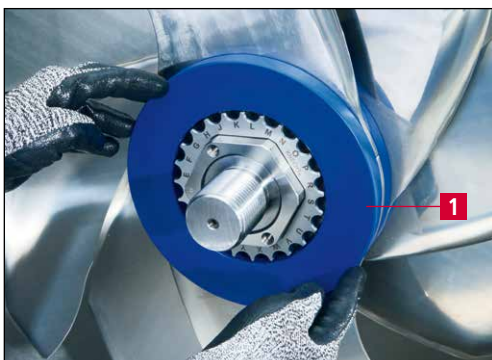
Figure 5-9 Assembling the knife package
