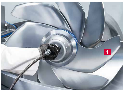
Figure 5-11 Installing the HSM 100 Hydro-mechanical clamping nut
