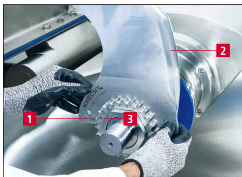
Figure 5-4 Installing the K24 Cutter knife
