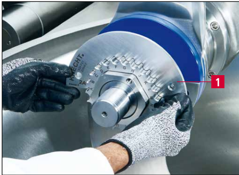
Figure 5-7 Installing the filling plate (FST)
