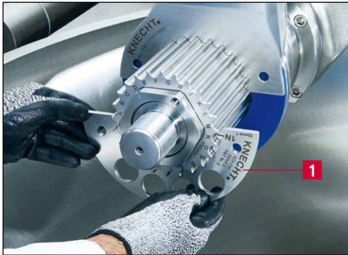
Figure 5-5 Installing the balancing filling plate (AWF)
