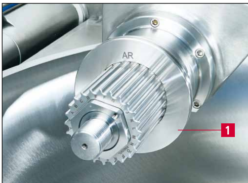
Figure 5-1 Installing the initial ring (AR)
