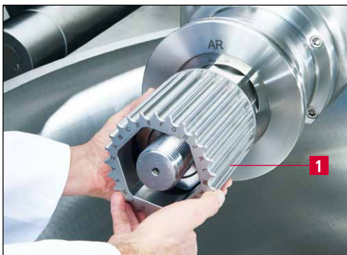
Figure 5-2 Installing the profile sleeve
