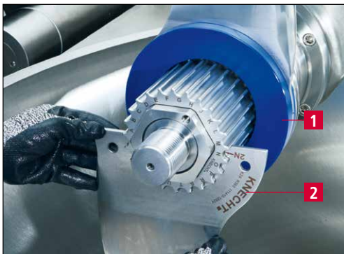
Figure 5-6 Filling plate (FST) installation
