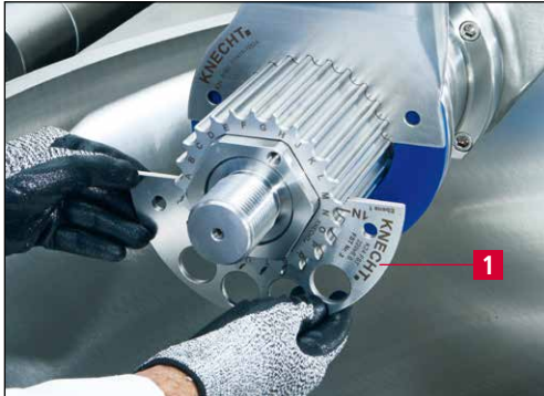
Figure 5-5 Installing the balancing filling plate (AWF)
