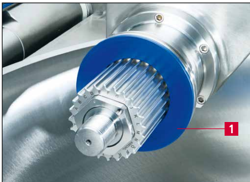
Figure 5-3 Installing the spacer ring (ZR)
