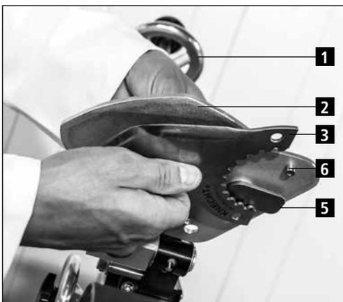
Figure 7-5 Tightening the cutter knife to the grinding plate
