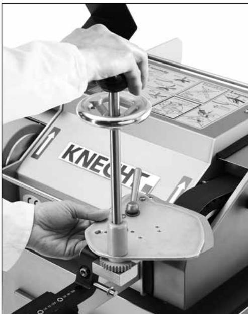
**Figure 7-12** Grinding the cutter knife
