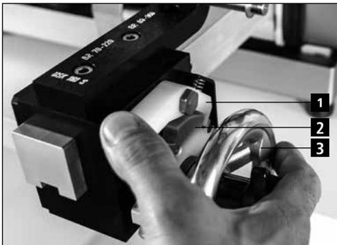
Figure 7-7 Turning the hand wheel to first locking position
