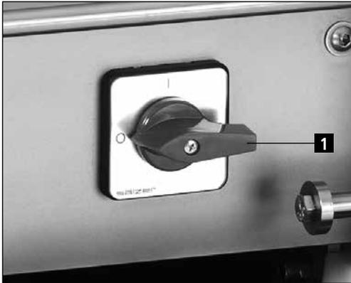
Figure 7-6 Switching on the grinding machine
