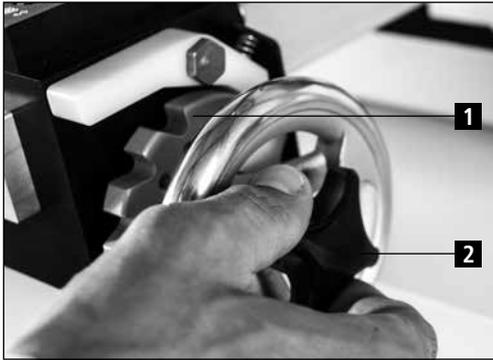
**Figure 7-8** Making the locking position inactive
