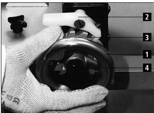
**Figure 7-7** Turning the hand wheel to last locking position
