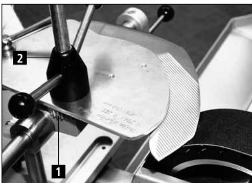
Figure 7-13 Inserting the function disk
