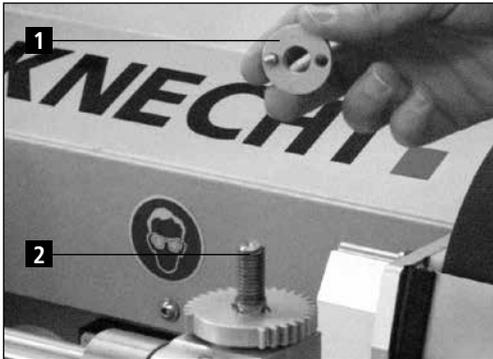
**Figure 7-3** Spacer disks for adjusting the grinding angle
