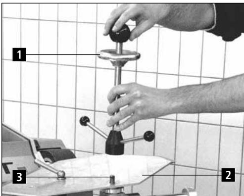
**Figure 7-5** Fix grinding plate with locking lever
