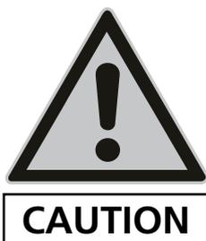
The hazard triangle with the signal word "CAUTION" is used as a work safety indication for all work which could result in death or physical injury.
