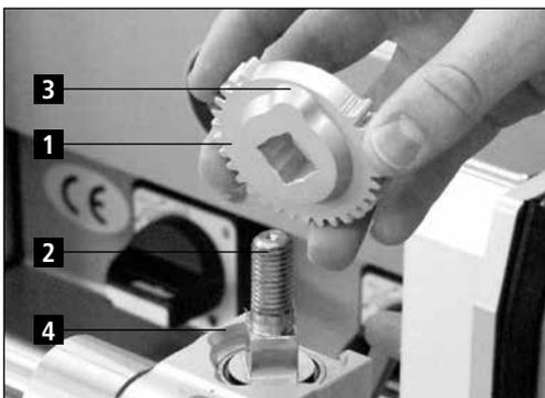
**Figure 7-2** Inserting the function disk
