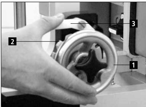
**Figure 7-9** Turning the hand wheel to second locking position.
