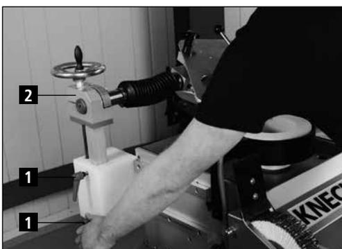
**Figure 7-21** Adjusting the cutter knife to the grinding wheel
