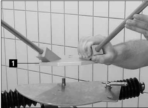
**Figure 7-3** Attaching the grinding lever
