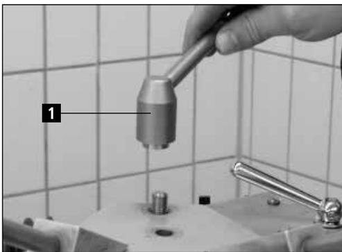
**Figure 7-4** Affixing the grinding plate
