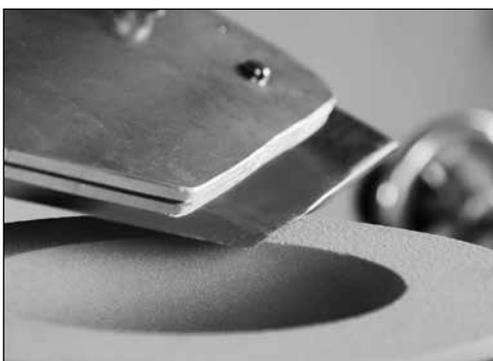
**Figure 7-9** Correctly configured knife
