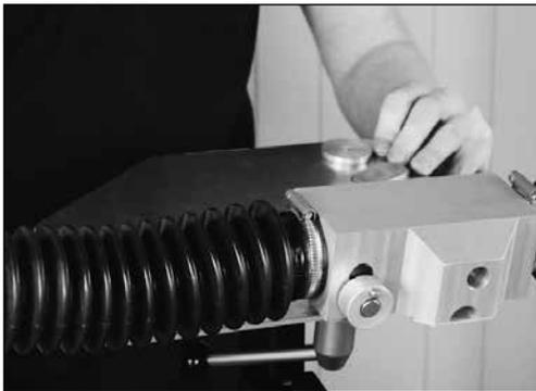
**Figure 7-5** Grinding plate in swiveled back position
