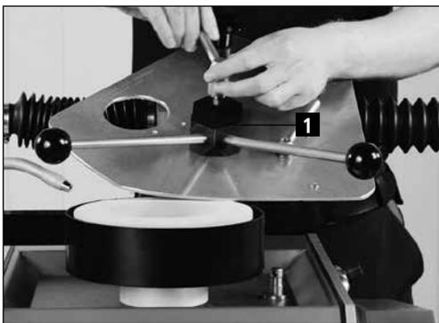
**Figure 7-18** Mounting the grinding lever
