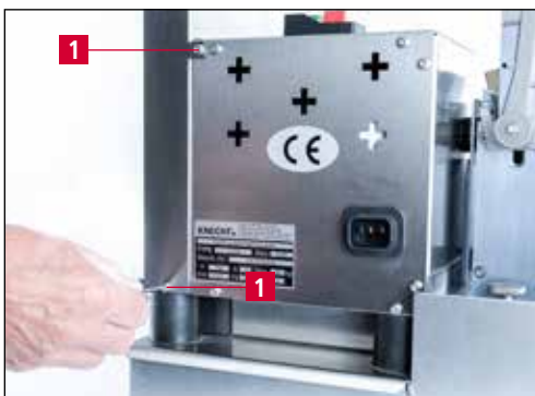
Figure 7-10 Loosening the polishing disk cover
