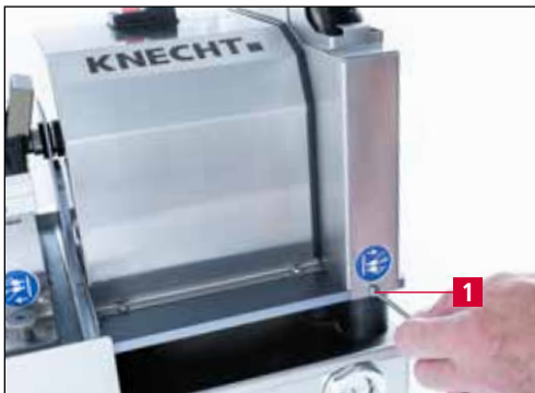
Figure 7-11 Loosening the polishing disk cover
