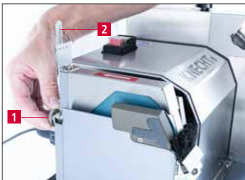
Figure 7-1 Adjusting the grinding angle
