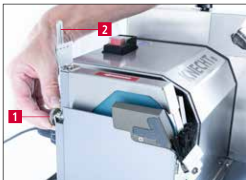
Figure 7-1 Setting the grinding angle
