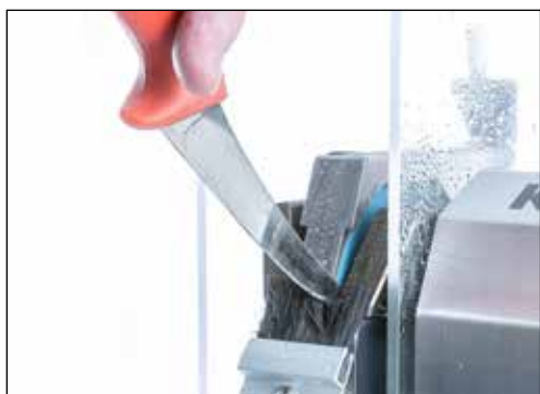
Figure 7-3 Sharpening hand knives
