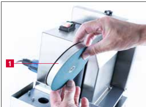
Figure 7-9 Installing a new pair of grinding wheels
