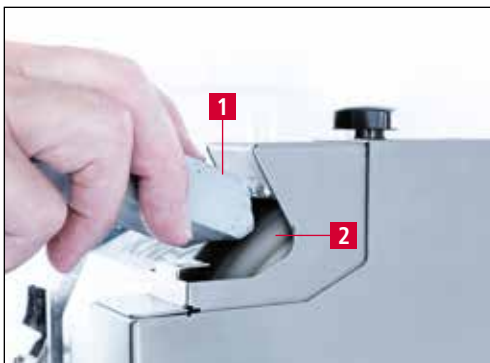
Figure 7-4 Applying the polishing paste
