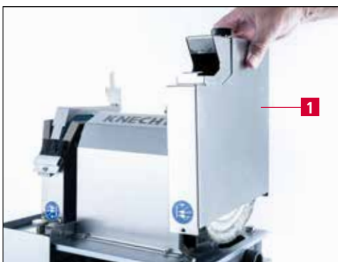
Figure 7-12 Removing the polishing disk cover
